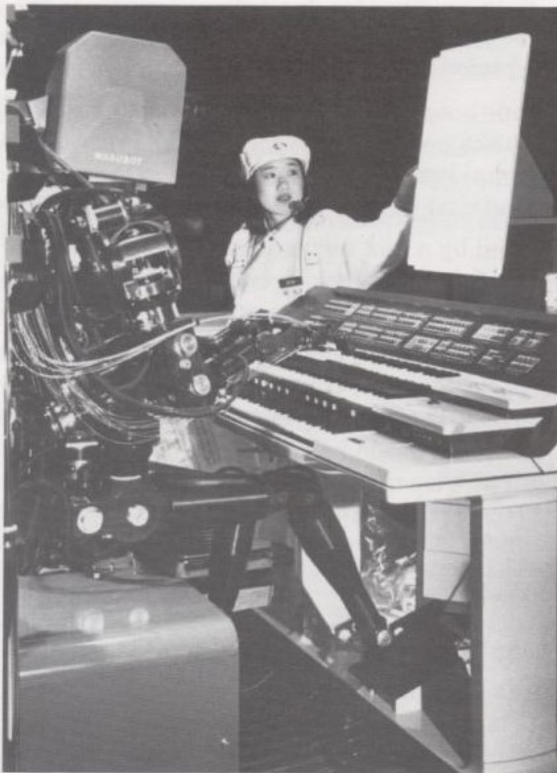
Japanese robot that plays organ and reads music through TV camera "eyes"
